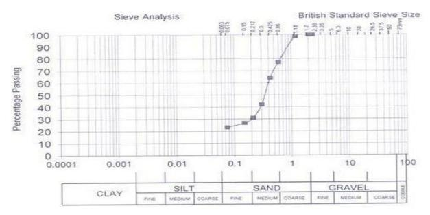
Figure 4. Typical particle size distribution curve.
